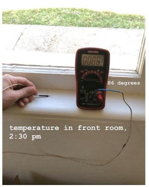
As you can see, this is nearly a 10 degree difference in the front room, and hours past when direct sunlight hits those windows. Given the severity in temperature difference, we believe that replacing the windows is the best solution.
